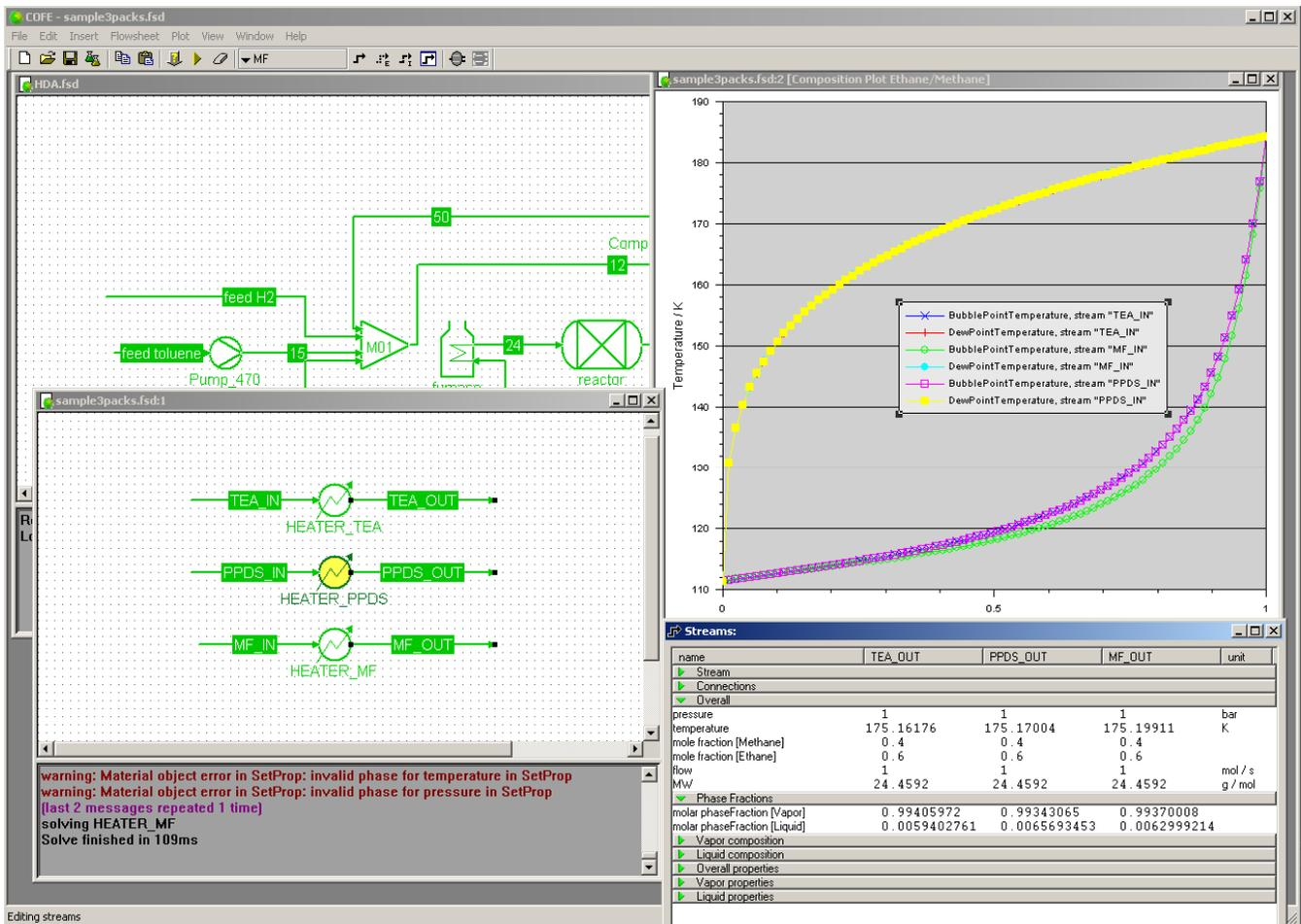
Figure 3: screenshot of COFE showing two open flowsheet documents. The document on top shows comparison of thermodynamic calculations of three different vendors. The stream view on the bottom right lists the results of the stream exiting the heaters (with equal configuration and equally defined inlet streams). The plot on the top right shows the phase envelopes for the three thermo systems at inlet stream conditions.
