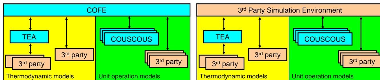
Figure 2: Schematic representation of simulation environments with thermodynamic models and unit operation models. All of COCO's components are exchangeable. Support for external models as indicated for third-party simulation environments differs from product to product.
