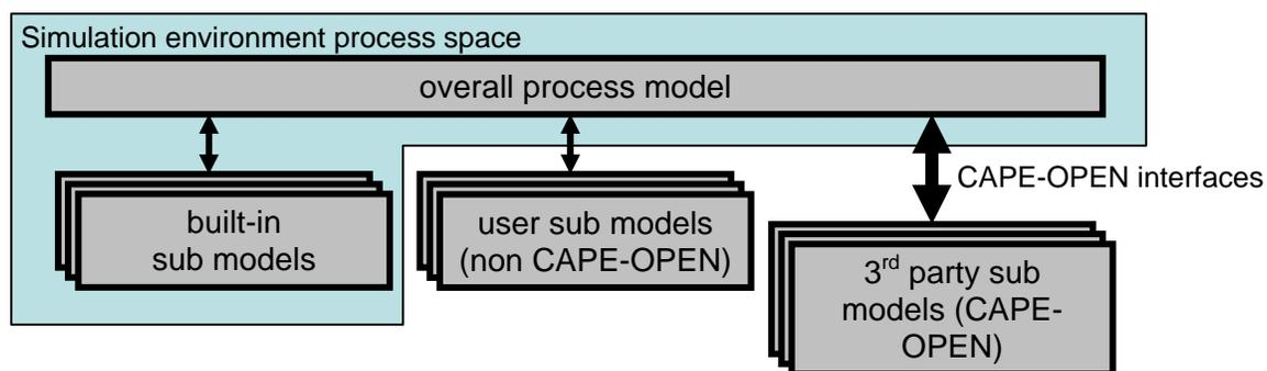
Figure 1: typical setup for process engineering modeling tools supporting CAPE-OPEN models.
